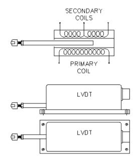
When the plunger is centered in its range the induced voltage of the two secondary coils is equal in magnitude, but opposite polarity. As the plunger moves to either side of the center position the voltage of one of the secondary coils increases while the other secondary coil experiences a decreased voltage. DC LVDT's differ from AC LVDT's in that they are manufactured with an internal carrier generator/signal-conditioning module and only require DC Power to operate.
